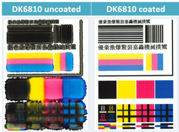
Figure 10: Inkjet printing results on film
